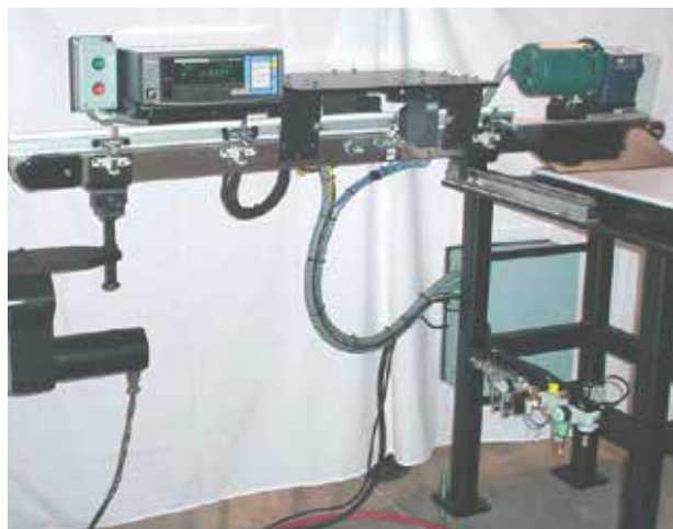
Post grind through-feed center-less shaft measurement
